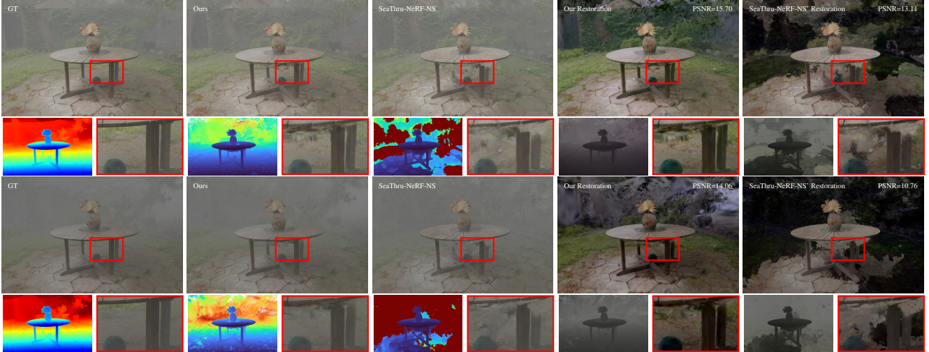
Figure 5. Simulated scene rendering with the easy foggy scene (upper) and hard foggy scene (lower). We compare our method with SeaThru-NeRF by showing both the full image and the rendering without the attenuation (restoration). Furthermore, under each image, we show the depth maps (for GT the depth map from pre-trained model [41]), and highlighted region from the image. For restoration, we further show the rendered medium without rendering objects. Our results exhibit better restoring quality and reasonable depth map compared to SeaThru-NeRF-NS’ results.
